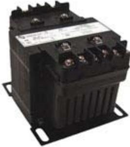
The HPS Emperor™ series of machine tool rated industrial control transformers are specifically designed to meet high inrush industrial applications where electromagnetic components such as relays, solenoids and magnetic motor starters are used.
